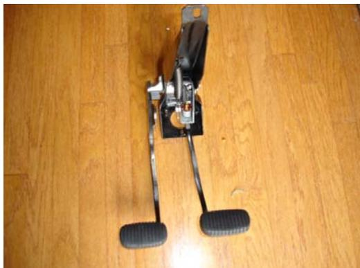
First thing I did was to paint every square inch of the pedals....to make sure rust never comes back. Then it was time to put the nylon inserts that go into the housing and provide a nice tight fit for the pedal axle. Uh oh....the insert did not want to go in...but I used force and finally got it in. Then it was time to put the clutch pedal in the insert. That was way too tight...but with more
