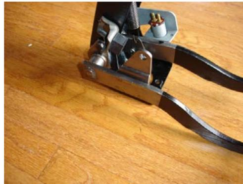
When I was done...in spite of a lot of WD40...I realized that the brake and clutch pedal had no movement at all.....unless you put quite a bit of force on it. There was no way that the brake pedal would go back and forth as intended. Oops.....it appears that the nylon inserts did not want all that protective paint in there.
