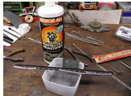
To replace the main blade holder segment, I started with used later production matte finish spade connector blades. I used a Dremel motor with a soft wire brush followed by hand sanding with 600 grit wet sandpaper and finished with polishing compound to achieve the desired
