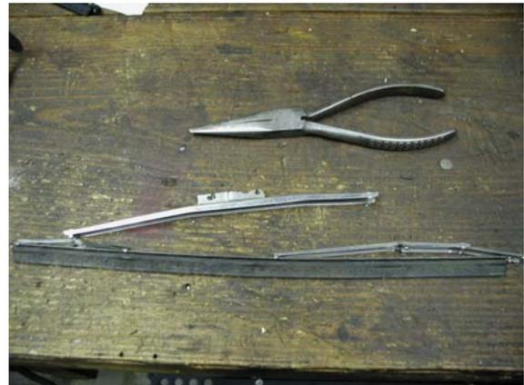
To help keep the rubber flexible, I treated them with Armor All using an old tooth brush.
