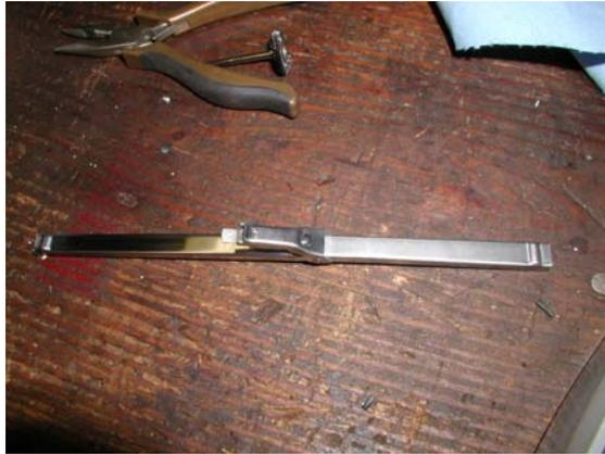
I removed the black plastic tips from old 11 inch and 15 inch blades. To put them on the new blades, it was necessary to use the Dremel motor with a cut-off wheel to make notches on each side and at both ends of the flexible metal strips (below).
