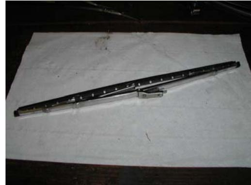
Closer inspection reveals "Can 63" stamped into the edge of the spade clip and "22" stamped into the main wiper holder segment directly beneath it. Also, unlike original parts, whose patent number stamping is completely on the unexposed portion of the end blade holder segments, the patent numbers stamped on the end blade holder segments of these extend past the attachment point and are partially visible adjacent to the Trico brand stamp.
