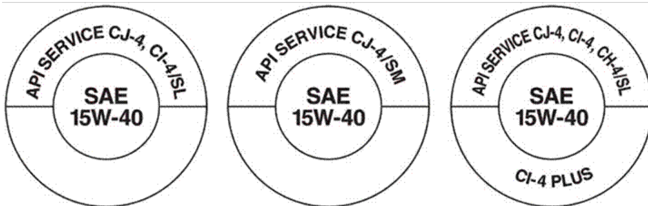
Typical primary category CJ-4 API service category symbols with various acceptable secondary categories. (Symbols courtesy of The American Petroleum Institute)
