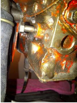
There is a hole on the side of the block.....that is threaded....so you can put a bolt in...and actually keep the rod up.....to enable you to insert the fuel pump. Much easier than trying to use your fingers....or need nose pliers.......
